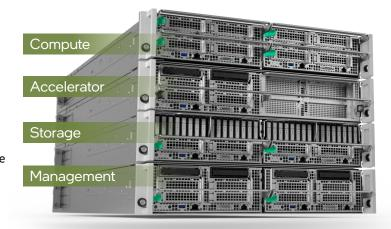
Storage module: Enables high density storage scalability for data-centric workloads, with up to 16 NVMe E1.L SSDs for up to 500 terabytes of storage capacity per module, along with two 3rd Generation Intel Xeon Scalable processors and two low-profile PCIe cards.
