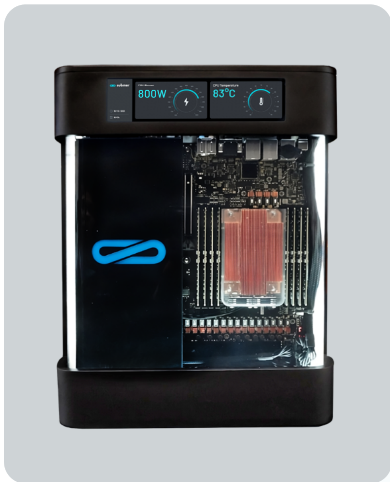
Figure 6 FCHS cooling overclocked Intel® Xeon® w9-3495X
